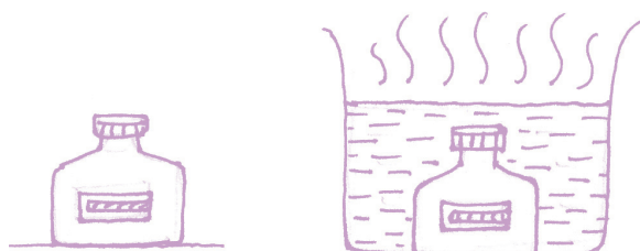
Fig. 14.9 Loosening a metal cap by heating it
