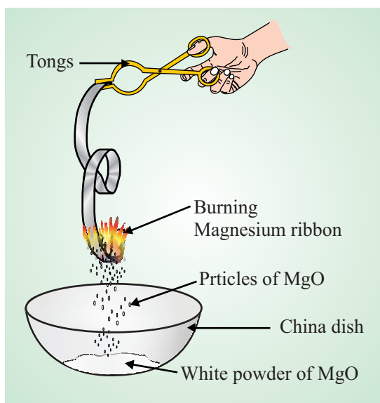
Fig. 4.1: Burning of magnesium ribbon
