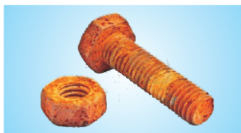
Fig. 4.9: Rusted nuts and bolts of iron
