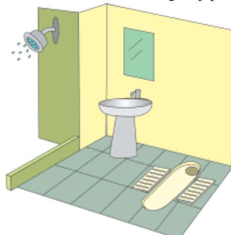
Fig.12.20: A squatting pan water closet
