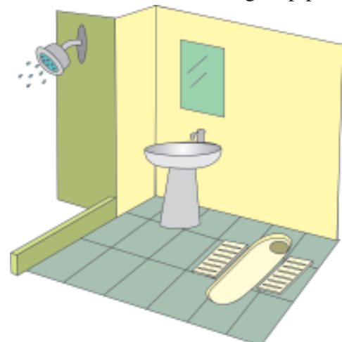
Fig.12.20: A squatting pan water closet
