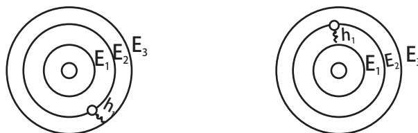
Fig. 2.11 : Absorption and emission of photon causes the electron to change its energy level.
