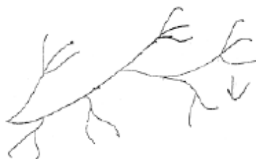
Fig. 31.2 : Branched chain polymers
