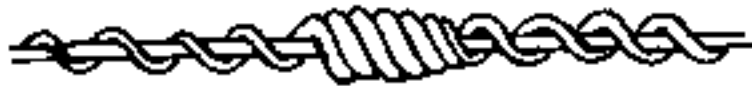
Fig. 23.8 : (f) KNOP – ground yarn is held under tension as knops are built up a fast speed
