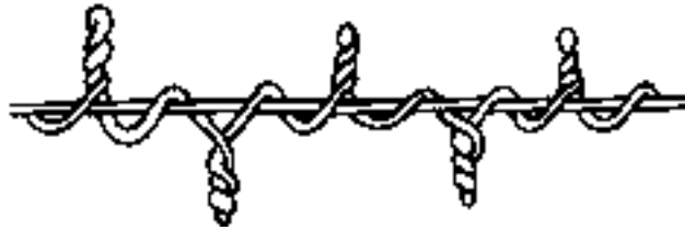
Fig. 23.8: (e) SNARL – very highly twisted yarn
