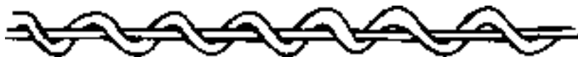
Fig. 23.8: (c) BOUCLE- two different yarns are fed into the loom at different speeds for a varied effect
