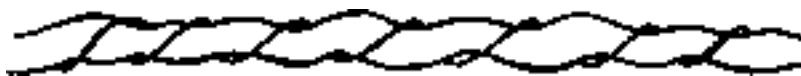
Fig. 23.8: (b) SPIRA or GIMP- combination of soft, thick yarns twisted with fine, hard yarns
